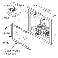
Figure 42 - Removing/Replacing Glass
